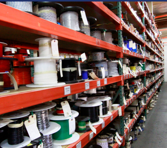
MIL-STAR aerospace-grade hookup wire is fabricated in accordance with AS22759 and AS27500 specifications. Complete baseline qualification test reports are available for all wire types as well as batch testing documentation on every production run.
