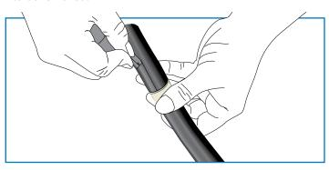
**C)** Beginning at the end of the wire, remove the scored insulation using needle nose pliers to gently pull insulation away, while working down the lengthwise incision and continue removing insulation from around diameter of wire. Once insulation is removed wire is ready for use.
