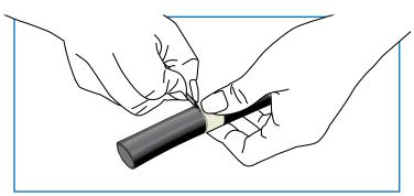
**B)** Proceed to score insulation lengthwise along the portion to be removed.
