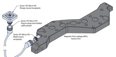
**◆** Application example shows the 707 Micro-PSI used to interconnect an MFL sensor to on-board PIG data storage.
