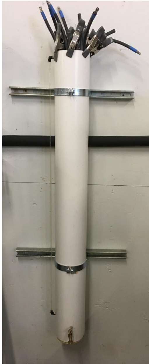
Image 2: Immersion insulation resistance tank.
