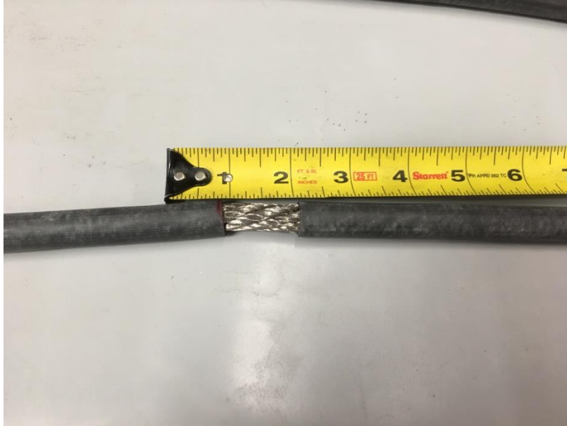
Image 3: 1 inch of section of Viton jacket material removed for Autoshrink installation.
