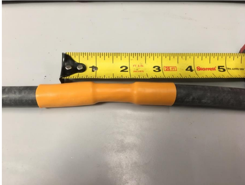
Image 4 : Example of Autoshrink installed on test sample over portion of removed cable jacket.
