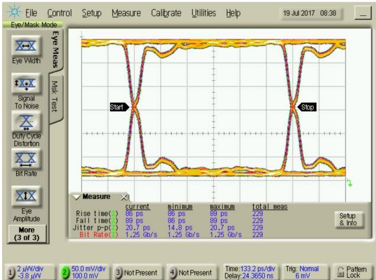
Figure 3: Eye diagram of GSGSG configuration at 1.25Gbps
