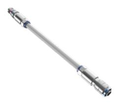
Lower installed cost. 100% tested. 10GbE. Save assembly time and cost with pre-wired SuperFly Datalink "White" assemblies for 10G Ethernet. These back-to-back Octaxial cordsets are terminated to Cat 6A aerospace-grade shielded cable. Two cable constructions are available: S/UTP (unshielded pairs with overall braid shield) or S/FTP (foil shielded pairs with overall braid). 24 AWG or 26 AWG stranded conductors. Series 882 connectors are designed for demanding aerospace environments.
