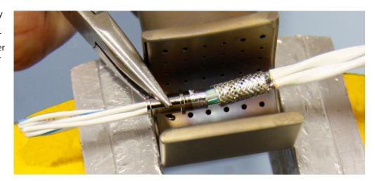
Next, grasp preform braid with needle nose pliers and return assembly to hot air gun reflector. When solder begins to melt, gently pull preform braid away from cable.
