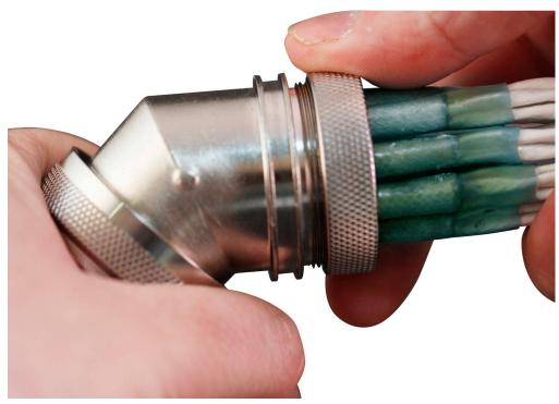
Tighten the gland nut on the body to the appropriate torque value.
