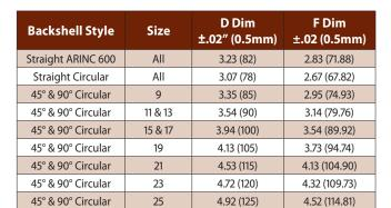
Strip the cables according to the following dimensions.
