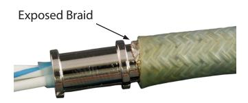
If solder has not completely melted and flowed within the preform assembly and/or outer heat shrink sleeve has not fully recovered, reheating may be necessary.
