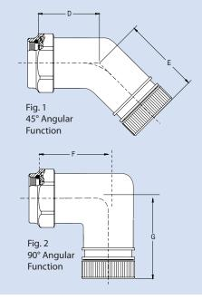
To calculate the cable length, see Table I (at left) to establish the *length constant* according to the connector designator's size and angular function. Then use the formula below to calculate the total length
