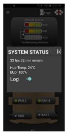
Tap the System Status Box and toggle the "Log" to allow for post mission analysis of power consumption. The "Log" will report the amount of power used enabling the proper battery choice for future missions.
