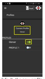
By default, the new profile will simultaneously become the "Current Profile," and be added to the list of available profiles. To change the "Current Profile" tap the corresponding profile toggle.
