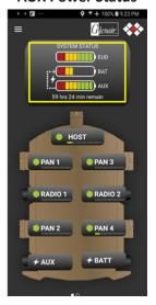
If an auxiliary power supply is connected to the STAR-PAN Hub, it is used by the system to charge the main battery, and individual port devices.
