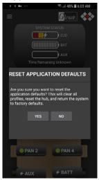
Upon tapping "Reset App Defaults" from the menu options screen, a pop-up alert confirming to clear all profiles, reset the hub, and return the system to factory defaults will appear. Select "Yes" to wipe all saved information and reset the hub.
