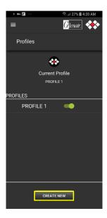
After tapping "Profiles" from the menu options screen the detailed profiles screen will appear. Select the "Create New" button to add a new profile.
