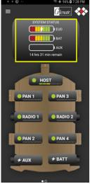
System Status Box shows charging hours and minutes remaining in EUD, and both BATTERY power supplies for use by all enabled devices attached to the hub (for SMBus-compatible batteries). Time will not consider peripheral device autonomy or radio battery sources connected w/ RPB.
