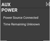
If the AUX power port is plugged to an AC power supply, the AUX power status bar will appear light gray and state "Time Remaining Unknown," since the source of the power supply is essentially unlimited.
