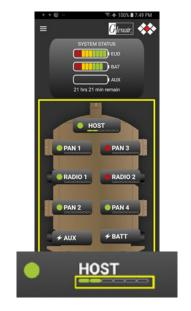
Enabled devices draw power. The amount is shown visually in a power load status bar directly under the port name.
