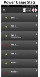
A second port-status "home screen" lists detailed battery power usage stats for all devices on the system. Note that you will only receive SMBus data if connected to a smart battery
