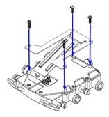
Remove and replace the two topmost screws, and the two screws second from the bottom using the following:
