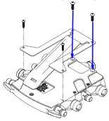
Position the MOLLE clip so the two larger screws are at the top of the hub.
