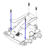
Remove and replace the two smaller screws second from the bottom using the following:
