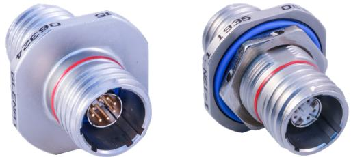
**SpeedMaster Glass-Sealed Hermetic:** Fully qualified to MIL-DTL-38999 Series III environmental and mechanical specifications.  $10^{-7}$  Helium leak rate. Outstanding high-speed performance. Bulkhead feed-thru shown.
