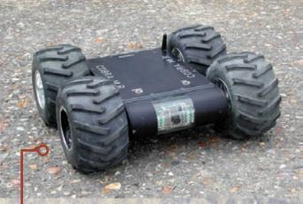
The ECA Inbot is controlled with a PDA or tablet PC and joystick. It is equipped with up to two hours of battery life and a  $\pm$  90° rotary head with color day/ night as well as infrared video.
