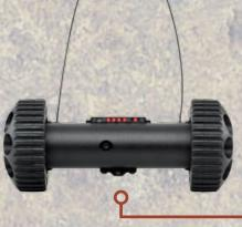
ReconRobotics Recon Scout IR tactical robot designed for tactical and SWAT applications, the man-packable and throwable MUGV is equipped with thermal/IR imaging and video broadcast capability.
