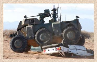
The Crusher is a 6,000 kg autonomous off-road UGV developed by Carnegie-Mellon University's National Robotics Engineering Center for DARPA. Optimized for rough terrain, the Crusher can easily overcome vertical walls, wooded slopes, and rocky creekbeds and carry 3,600 kg of armor and cargo.
