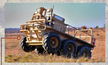
Lockheed-Martin Squad Mission Support System (SMSS), designed for transport and logistics support, is the largest UGV ever deployed with US forces.
