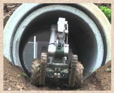
Going where soldiers don't want to go: the Cobham Telemax UGV is designed for use in confined spaces and/or overcoming tall obstacles and varied terrain
