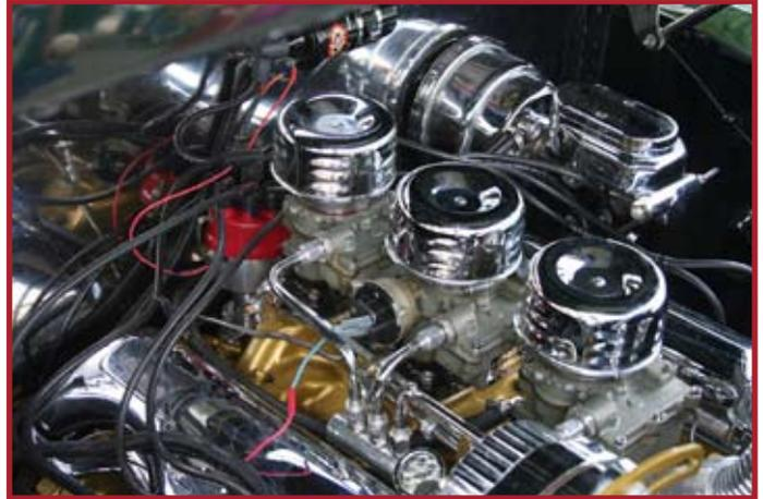
***Under-the-hood wiring is frequently a combination of insulated wire bundles, jacketed cables and polymer plastic convoluted tubing used to protect circuits subject to heat or abrasion damage. In late model engine applications, under-the-hood temperatures are considerably higher and often require the use of special high-temperature conduit materials to effectively protect wire circuits.***
