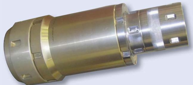
***Special strain-relief backshell invented by Glenair for use on the French TGV rail system. This backshell design resolved complex intercar vibration and shock problems which resulted in destructive cable damage.***
