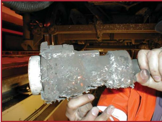
**Connectors and cables see tough, environmental duty in rail applications. Poorly sealed products, or those made from inappropriate materials, can lead directly to system failures.**
