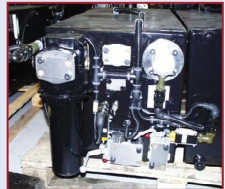
Conduit harnesses on some U.K. locomotive oil reservoirs included multiple fittings and sharp bends to fit properly on the equipment. With constant vibration and high temperatures, the conduit failed
