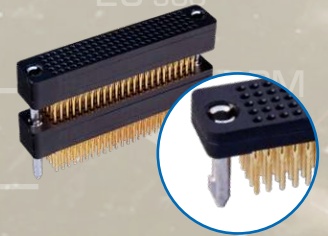
Polarized shells and keyed guide pin hardware prevent mis-mating
