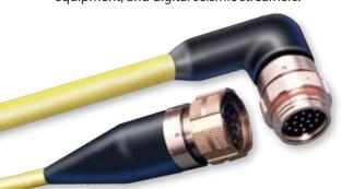
Geo-Marine® plugs are equipped with arctic coupling nuts—made from marine-grade naval bronze with easy-to-grip castellated knurling and a powerful ratcheted anti-decoupling mechanism which guarantees reliable mating and demating performance in even the harshest environments. Supplied as discrete connectors or more typically in build-to-print overmolded cable assemblies.
