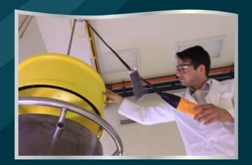
SeaKing™ and SuperG55™QUALIFICATION TESTING: Both Glenair Series 70 SeaKing and SuperG55 rugged dry-mate subsea connectors have been tested and qualified to their 10K psi pressure rating—open-face and mated—in Glenair's state-of-the-art hydrostatic test lab. Additional testing included mating cycles, salt spray, and electrical continuity
