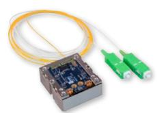
RF-over-fiber board-mount transceiver
