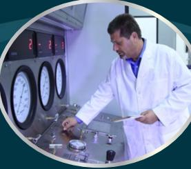
5. Small connector pressure test bunker
