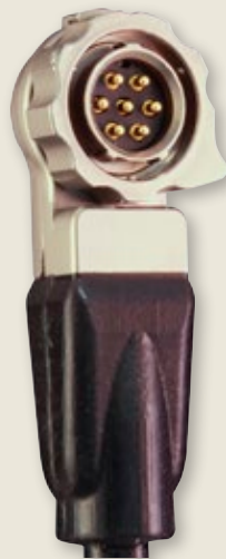
The Series 807 Mousebud™ is a lightweight, low-profile, quick-disconnect connector optimized for rugged applications. Available in plug and receptacle configurations, the spring contact equipped Mousebud™ is a 7-channel, 3 amp per line solution for such applications as heads-up display helmet applications, soldier computers and field communications equipment. The Mousebud™ has a spring-loaded latching mechanism that connects with a simple push, and releases with a low-profile thumb-activated lever on the plug coupling nut. Split-shell plug design provides easy access to wire terminations and an integrated banding porch eliminates the need for additional backshell accessories. Environmentally rated to IP67, the Mousebud™ is ready for application in a wide range of harsh environments.
