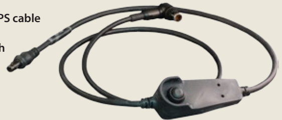
The Series 807 Mousebud™ is a lightweight, low-profile, quick-disconnect connector optimized for rugged applications. Available in plug and receptacle configurations, the spring contact equipped Mousebud™ is a 7-channel, 3 amp per line solution for such applications as heads-up display helmet applications, soldier computers and field communications equipment. The Mousebud™ has a spring-loaded latching mechanism that connects with a simple push, and releases with a low-profile thumb-activated lever on the plug coupling nut. Split-shell plug design provides easy access to wire terminations and an integrated banding porch eliminates the need for additional backshell accessories. Environmentally rated to IP67, the Mousebud™ is ready for application in a wide range of harsh environments.
