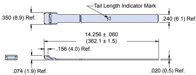
The 600-052 Standard Band is precision constructed of 300 Series SST/Passivate and designed for use with the 600-058 Hand Banding Tool or the 600-067 Pneumatic Banding Tool. Double-wrapped bands will accommodate diameters up to approximately 1.8 inches (45.7). Bands may be ordered flat (600-052) or precoiled (600-052-1). Bands come bagged and tagged in quantities from 1 to 100.
