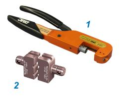
Parallel action tool for use with hex crimp dies. 11 inches OAL, 2.0 pounds. Anodized aluminum frame, steel mechanism, plastic handles. Includes tool for die set removal. Accepts all M22520/5 die sets.
