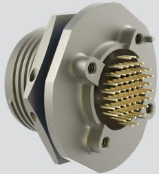
*Ceramic planar array C and Pi filters. Jam-nut panel mounting. PC tail with board mounting flange.* 240-806-21 filtered receptacles save size and weight compared to legacy aerospace-grade EMI/RFI filter connectors. These high-performance connectors are suitable for areas subject to high vibration, altitude, and moisture as well as temperature ranges from -55°C to +125°C. Size 20HD and size 22HD contacts. Board mounting flange has threaded standoffs and orientation post.
