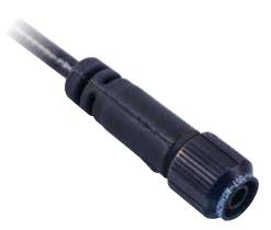
Harsh Environment Cordsets Overmolded Series 811 cordsets withstand abrasion and chemical exposure. Cable construction features silver coated stranded conductors with TFE insulation, tinned copper braid shield and extruded black polyurethane jacket. Choose single-ended pigtails or double-ended "back-to-back" cables. Semi-rigid polyamide overmold provides strain relief and environmental sealing.
