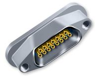
**Glenair's Hermetic Micro-D Connectors** feature fused glass insulators to provide an airtight seal. These connectors are 100% tested to meet a maximum leak rate of 1 X 10<sup>-7</sup> cc's per second of helium.
