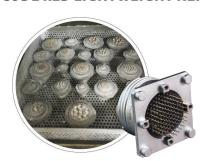
Connectors utilizing CODE RED hermetic encapsulant sealing went through a grueling qualification test and validation process to prove material durability and hermeticity. Validation testing including 100 cycles of thermal shock IAW EIA-364-32 Test Condition A -65°C to +200°C while maintaining hermeticity followed by 1000 hours of thermal aging at 200°C. Additional tests included:
