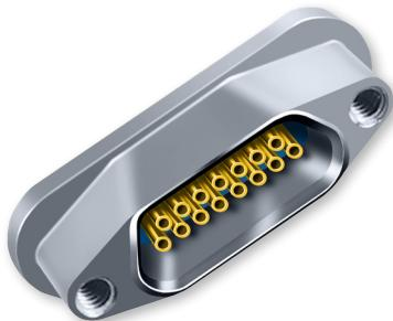
**Glenair's Hermetic Micro-D Connectors** feature fused glass insulators to provide an airtight seal. These connectors are 100% tested to meet a maximum leak rate of  $1 \times 10^{-7}$  cc's per second of helium.
