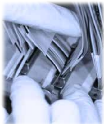
Potting a Micro-D with Epoxy-Filled Syringe
