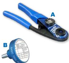
Precision mil spec crimp tool performs precision eight indent crimps for gas-tight wire terminations and excellent tensile strength. Adjustment wheel has 8 settings. Ratchet mechanism prevents improper crimps. Use with bayonet-type positioners, ordered separately. Check calibration with M22520/3 gages. Length is 6.75 inches, weight is approx. 10 oz.
