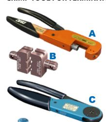
A Parallel action tool for use with hex crimp dies. 11 inches OAL, 2.0 pounds. Anodized aluminum frame, steel mechanism, plastic handles. Includes tool for die set removal. Accepts all M22520/5 die sets.
