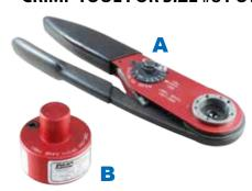
Heavy-duty M309 crimp tool for AWG size 8 to 18 wire. Adjustment wheel has 8 settings. Double action ratchet mechanism prevents improper crimps. Use with positioner, ordered separately.
