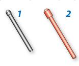
Grommet sealing plugs are used to seal unwired contact cavities. These plugs conform to MS27488 requirements. After installing unwired contacts into unused cavities, insert knob end of sealing plug into grommet until it bottoms against the unwired contact per illustration. Install sealing plugs with standard contact insertion/extraction tools .
