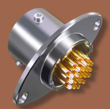
Series 80 Mighty Mouse Hermetic Mighty Mouse Hermetic Receptacles feature stainless steel shells and Alloy 52 iron alloy contacts. The compression glass seal is rated at 1 X 10<sup>-7</sup> cc/second helium leak rate. Coupling styles include doublestart stub acme, quick disconnect and bayonet.
