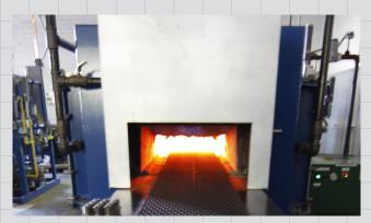
The connectors enter the furnace on a conveyor belt and a gastight hermetic seal is formed around all contacts, and between the glass seal and the connector shell, when the vitreous glass is melted in the furnace and then cooled under controlled conditions.
