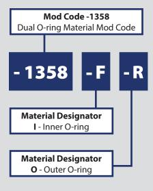
Mod Code 1358 can be added to to any part number of any connector with dual O-ring flanges to specify an alternate material better suited for a specific applications.
