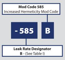
An array of hermetic connectors with more stringent leak rate requirements. By adding "**-585**" and the designator letter "**A**", "**B**", "**C**", "**D**"—depending on the hermeticity desired—to the end of a standard part number, connectors will be built to exceed the standard 1 x 10<sup>-7</sup> cc Helium per second leak rate specified on most Glenair hermetics.
