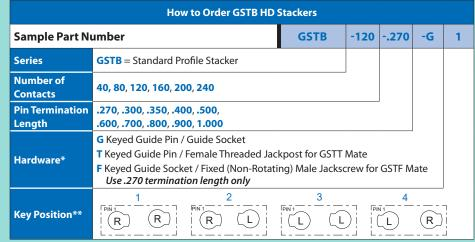
$\star$  For **T, F** hardware, connectors with 40 to 160 positions have #2-56 threads, connectors with 200 to 240 positions have #4-40 threads
