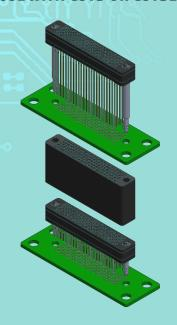
Glenair supplies nine standard spacers ranging from .030" to .730" (.76mm to 18.54mm) to allow application designers to engineer board-to-board heights ranging from .295" (no spacer) to 1.025" (7.49mm to 26.04mm). Dielectric spacers also serve to insulate free-standing connector pins, and act as rigid standoffs in board-to-board applications.
