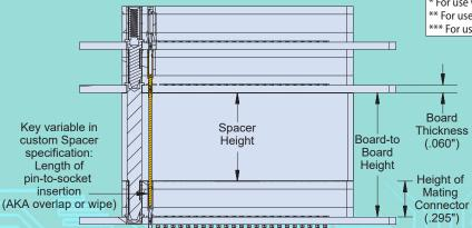
Illustration left depicts all of the standard variables affecting board-to-board height. While custom spacers are available, care must be given to ensure pin termination lengths result in adequate pin-to-socket overlap (not to be reduced in excess of .100")
