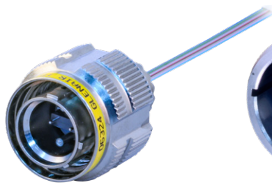
Plug with EMI/RFI ground spring Shell size-insert arrangement 11-1, Up to 24 fibers (1 MT ferrule)
