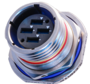
Jam nut receptacle Shell size-insert arrangement 17-4, Up to 96 fibers (4 MT ferrules)
