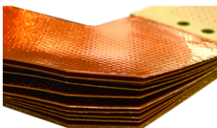
Multilayer rigid-flex circuit assemblies—up to 27 layers—offer increased circuit density while still maintaining the medium's dynamic 3D flex characteristics
