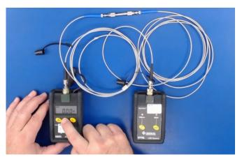
**4.** Attach test probe adapters to connectors and insert test probes into corresponding pin and socket.
