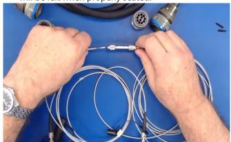
**3.** Zero out test probe adapters by pressing and holding the button labeled dB/dBm. Readout is in dB.
