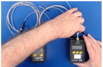
**2.** Insert probes into calibration adapters. Tactile click will be felt when properly seated.
