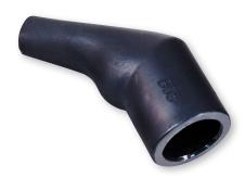
Lipped, 45° angle heat shrink boots provide mechanical and environmental protection from damage and debris. These shrink boots fit most standard boot adapters for circular connectors. All adhesive lined and unlined shrink books are RoHS compliant. Shrink boots are water-tight when equipped with factory installed or user-installed adhesive. Lipped boots lock into boot groove located on adapter. Choose boot size based on adapter diameter and cable diameter.
