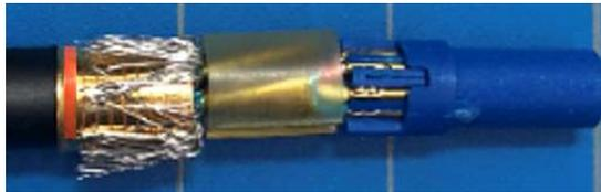
**Inspection Step:** the gap between the plastic bushing and the adjacent component shall be less than 0.010”.
