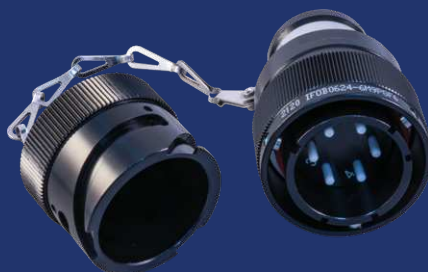
SUPER ITS-IFO B FIBER OPTIC CONNECTORS 6-Pole fiber optic, shell size 24 connector with environmental sealing PG backshell for conduit termination or PGSW backshell with strain relief for use with jacketed cables
