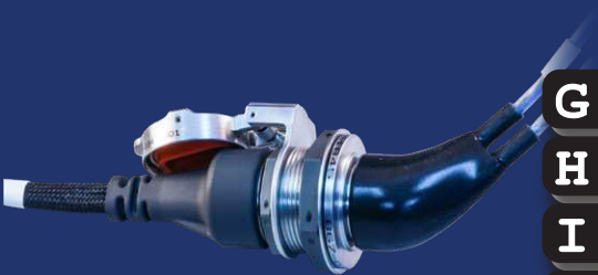
Mated GateLink Pro™ plug and receptacle cordsets with shielded twisted pair cabling. Plug side features environmental overmolding, receptacles side utilizes strain relief boot
