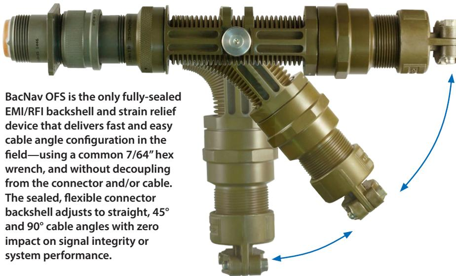
BacNav OFS is the only fully-sealed EMI/RFI backshell and strain relief device that delivers fast and easy cable angle configuration in the field—using a common 7/64" hex wrench, and without decoupling from the connector and/or cable. The sealed, flexible connector backshell adjusts to straight, 45° and 90° cable angles with zero impact on signal integrity or system performance.
