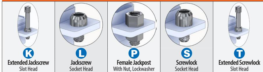
Screwlocks allow connector to be plugged in before the screws are tightened. Jackscrews must be tightened in order to mate connector.
