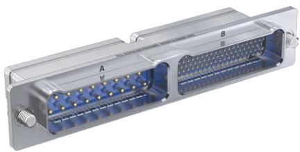
**Dual bay cable mount.** Space-saving 793-017 connector features high-density, high current and high frequency capabilities, saves size and weight compared to legacy rack-and-panel types. Connector has two inserts. Machined scoop-proof shell has groove for attaching backshell. Size 23 contacts are included with connector; size 8, 12, and 16 contacts are ordered separately. Connectors become non-scoop proof at parallel horizontal angles of entry from 16°–47°.
