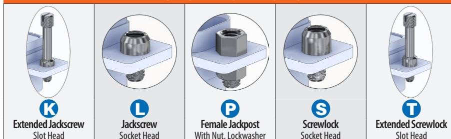
Screwlocks allow connector to be plugged in before the screws are tightened. Jackscrews must be tightened in order to mate connector.
