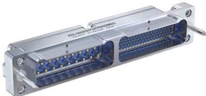
**Dual bay blind mating.** Space-saving 793-002 receptacle features high-density, high current and high frequency capabilities, saves size and weight compared to legacy rack-and-panel types. Machined scoop-proof shell has groove for attaching backshell. Size 23 contacts are included with connector; power contacts (#8, #12 or #16) or coaxial RF contacts (#12 and #16) are ordered separately. Connectors become non-scoop proof at parallel horizontal angles of entry from 16°–47°.
