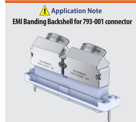
Use backshell part number 799-015 (Size M). Two backshells are required per connector. Two piece backshell has lip to lock into groove on connector. Available in top entry, side entry and 45° entry.
