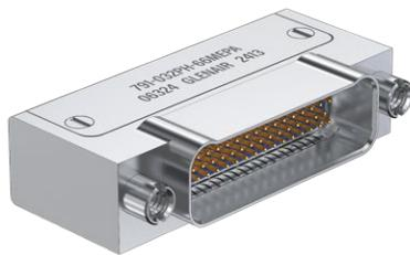
791-032 receptacle has right angle PC tails for thru-hole printed circuit board termination. Contacts are sealed with epoxy. Machined aluminum shell has integral standoff and threaded holes for attachment to PC board. Fluorosilicone seal provides environmental protection to mating interface. Available in forty insert arrangements with up to 102 contacts. Contact sizes include high-density #23 contacts on .075 inch (1.9mm) centers, #16 contacts, #12 contacts, and #8 contacts.
