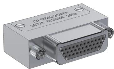
791-016 plug has right angle PC tail socket contacts for thru-hole printed circuit board termination. Contacts are sealed with epoxy. Machined aluminum shell has integral standoff and threaded holes for attachment to PC board. Available in forty insert arrangements with up to 102 contacts. Contact sizes include high-density #23 contacts on .075 inch (1.9mm) centers, #16 contacts, #12 contacts, and #8 contacts.
