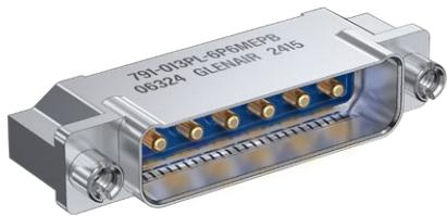
791-013 receptacle has straight PC tails for thru-hole printed circuit board termination. Contacts are sealed with epoxy. Machined aluminum shell has integral standoff and threaded holes for attachment to PC board. Fluorosilicone face seal provides environmental protection. Available in forty insert arrangements with up to 102 contacts. Contact sizes include high-density #23 contacts on .075 inch (1.9mm) centers, #16 contacts, #12 contacts, and #8 contacts.
