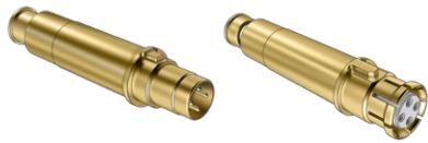
Quadrax contacts are used for 100 Mbit/s Ethernet protocols including 100BASE-TX and ARINC 664. Crimp termination. Supplied as unassembled kit with sealing boot and instruction sheet. Contacts snap into connector body and are removable with plastic tool purchased separately.
