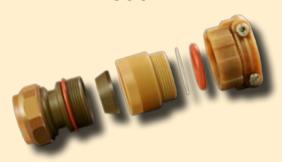
Glenair's composite Series 390 backshells utilize standard cone and ring style shield termination to deliver 360° shield/screen grounding with low DC resistance across the termination area. Cable sealing O-rings provide full-immersion protection to 6 ft. The lightweight, corrosion proof backshell is ideally suited to general duty use in both military and commercial interconnect cable applications. Glenair 390 series backshells are fully tooled for all popular connector series and sizes.
