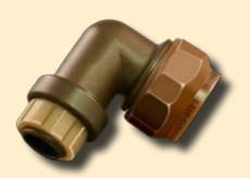
A sleek, compact shield termination backshell assembly that utilizes a simple lamp-base thread device to capture conductive cable shielding; yielding both strain relief and EMI/RFI protection. Straight and 90° shell styles are available. This simple, light-weight backshell may optionally be equipped with a shrink-boot for a modicum of environmental protection.
