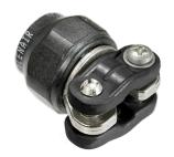
Self-locking. Full radius saddles. Lightweight, corrosion-proof composite saddle clamp fits Glenair Series 806 MilAero connectors. For use with open bundle wiring harnesses and closed bundle (jacketed) harnesses. Anti-decoupling mechanism provides audible detented coupling and prevents backoff under high vibration. Telescoping screws. Full radius saddles are intended to be bottomed onto frame. High temperature thermoplastic. Straight, 45° and 90° profiles.
